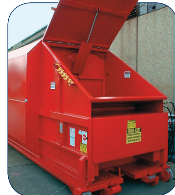
Optional hydraulically operated lid for 265X-WQ can be used to restrict unauthorized access and limit exposure to the elements.
