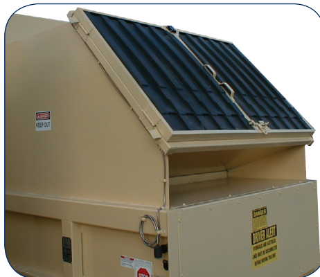
Crossed cylinder design and extended rear feed hopper allows customer to load this unit from a dock door without ever leaving the dock. (Shown here with plastic lids & interlock)
