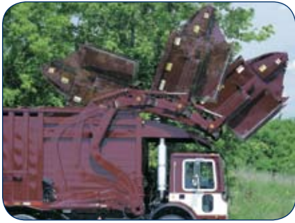
Spring assisted compactor lid
